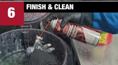
Remove masking tape while final coat is still wet. Clean gun with XXX Universal Gun Cleaner or solvent complaint with VOC regulations in your area.
