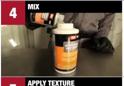
Add activator to bottle of **2K Urethane Chip Guard**. Shake bottle for two minutes before applying.
